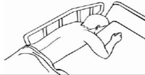
Zone 5 – Entrapment between split bed rails
