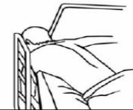
Zone 6 – Entrapment between the end of the rail and the side edge of the head or foot board
