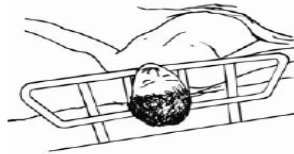
Zone 3 – Entrapment between the rail and the mattress
