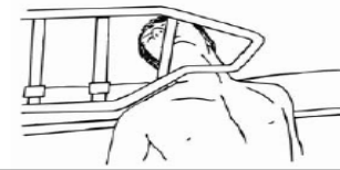
Zone 6 – Entrapment between the end of the rail and the side edge of the head or foot board
