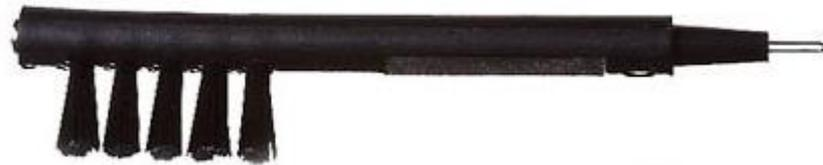
← Wire tip can remove wax safely
